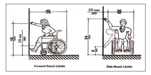
Below is a chart listing each MC cabinet model and the corresponding **MAX INSTALLATION HEIGHT** necessary to comply with the ADA requirements. The measurement shown is taken from the base (bottom) of the machine to the floor. Additionally, ADA requires a 30" (760mm) by 48" (1220mm) "clear floor space" to provide sufficient clearance for a single wheelchair and occupant.
