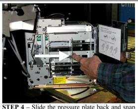
**STEP 4** – Slide the pressure plate back and snap into position.
