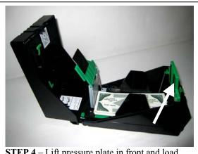
**STEP 4** – Lift pressure plate in front and load bills.
