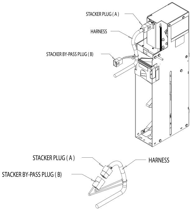
To operate the machine without a stacker, follow the steps below:
