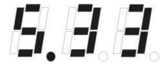
The display is only a single digit; therefore, to obtain the 3-digit error code the first digit is displayed WITH THE DECIMAL POINT (5.) and the second and third digits are displayed WITHOUT THE DECIMAL POINT (3) (3). The display will continue to flash the 3-digit error code; one digit at a time, until the failure is corrected or power is removed.
